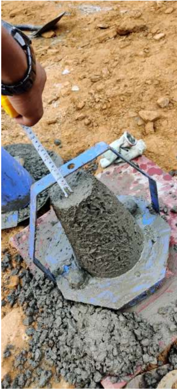
Picture 20: Slump test and Concreting of Columns of Lower ground floor of Grid 5
